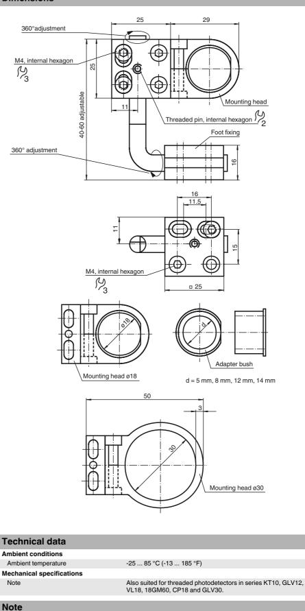
The mounting adapter is supplied with 2 mounting heads (ø18 mm, ø30 mm) and 4 adapter bushes (ø5 mm, ø8 mm, ø12 mm, ø14 mm).
