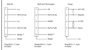
According to the "PROFIBUS Mounting Recommendations", the connection of the screen with Pin 5 is not recommended. If necessary, this type connection should be chosen if the contact of the screen cannot be established by screwing it to the plug housing.
