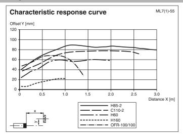
Retroreflective sensor with polarization filter
