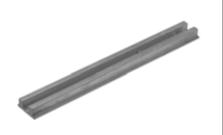
Connectors are necessary for joining the aluminium profile rails. Each connector (WCS3-MC1) consists of a 170 mm long aluminium extruded section and two selftapping screws M3 x 4.5 mm. The connector is pushed into the bottom grooves in the two profile rails to be joined. Then the screws are screwed into the holes (1.8 mm in diameter). The tips of the screws are pressed into the aluminium profile and hold the connector down.
