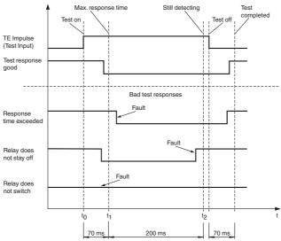
The door controller must query the sensor at times t<sub>1</sub> and t<sub>2</sub>.
