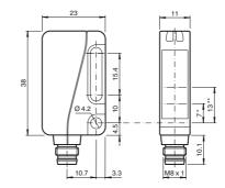
\* optical axis transmitter \*\* optical axis receiver
