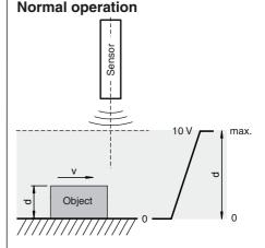
In normal operation, the sensor outputs a value at the analog output, which is proportional to the thickness of the object. The object thickness 0 mm (measurement to the reference object) is represented in this by the minimum analog value and the largest measurable object thickness (see Technical Data) is represented by the maximum analog value.
