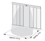
Installation height 2200 mm / angle of detection field  $30^{\circ}$
