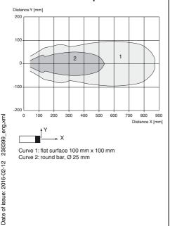
Curve 1: flat surface 100 mm x 100 mm Curve 2: round bar, Ø 25 mm
