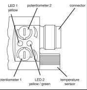
The potentiometer function described illustrates the default function. The function of the potentiometer can be altered using the ULTRA-PROG-IR software. As soon as a configuration has been changed, the potentiometer function selected using ULTRA-PROG-IR is activated.
