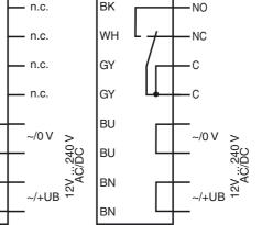
The relay-functions "NC" and "NO" bear on the switching mode "Dark-ON". This complies to the default setting of the light/dark switch (factory setting).
