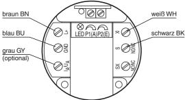
The terminals I<sub>A</sub>/U<sub>A</sub> (analog output) and SX (2<sup>nd</sup> switching output) are not needed for programming.
