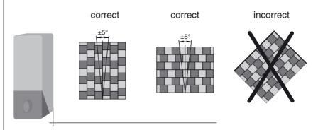
The edge of the sensor must be parallel with the edge of the reflector!
