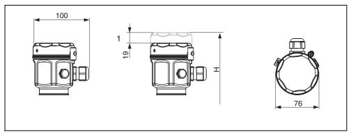
1 The cover with viewing window is 19 mm (0.75 in) higher than the cover without viewing window.
