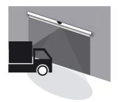
\*) Vehicles crossing the detection range of the sensor may cause the human-presence relay to be activated unexpectedly.
