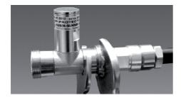
Coupling nut torque must not exceed IEC standard or manufacturer specifications (IEC: max. 1.13 Nm). The bending moment created by connected cables must not exceed 1 Nm.
