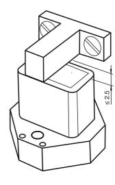
panel of the sensor) and the fixing base or fixing elements (e.g., protruding screw heads) of the actuator must be at least 10 mm.
