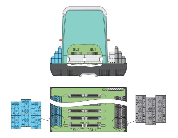
Insert the isolated barrier on the Termination Board. This closes the signal circuit between field side and control side. Connect field devices and controller to the terminals or connecting plugs of the Termination Board. For pin assignment between terminals, connecting plugs and connectors SL1/SL2, see drawing "Connection diagram" or the corresponding pin-out table on www.pepperl-fuchs.com.
