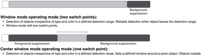
• Detection of objects irrespective of type and color in a defined detection range. Sets a defined window around a given object. Objects outside this window are not detected.
