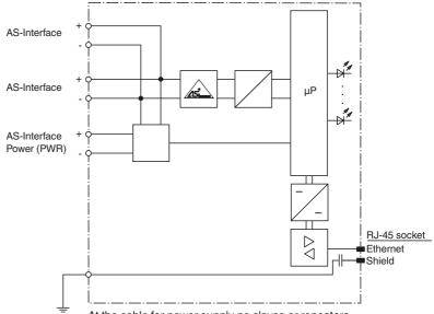
At the cable for power supply no slaves or repeaters may be attached.
