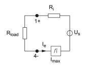
$$\begin{split} R_{load} &= Field \ \text{loop resistance} \\ U_e &= U_s - R_i \ x \ I_e \\ I_e &= U_s / (R_i + R_{load}) \end{split}$$
