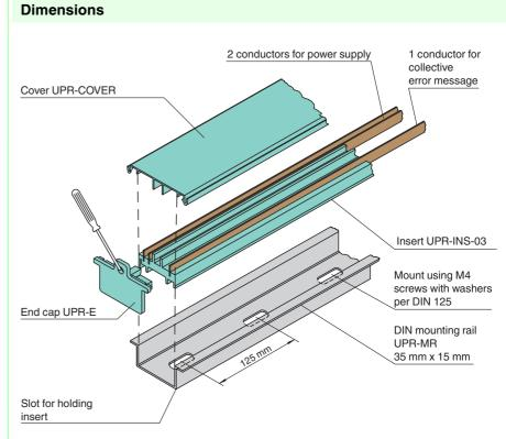
Universal Power Rail with end caps and cover, 3 conductors, length: 1,6 m
