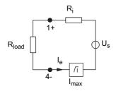
$\begin{aligned} &R_{load} = \text{Field loop resistance} \\ &U_e = U_s - R_i \times I_e \\ &I_e = U_s / (R_i + R_{load}) \end{aligned}$
