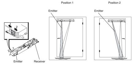
The transmitter of each sensor features two beam position settings via which the monitoring edge can be aligned to the left or to the right.
