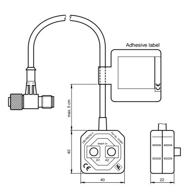
The unit can be switched from the V15 cable connection socket and the V15 plug connection on the sensor for the TEACH-IN procedure.
