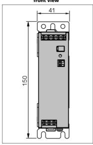
Fig. 22-5 Hole pattern for wall mounting
