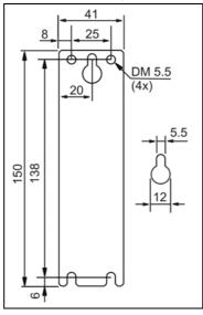
Fig. 22-6 Wall/panel mounting, side view
