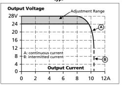
Fig. 6-2 **Dynamic output current capability, typ.**
