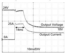
Please note: The DC-OK relay triggers when the voltage dips more than 10% for longer than 1ms.
