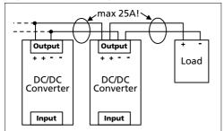
Fig. 13-2 Using distribution terminals
