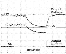
Fig. 23-2 41.5A peak current for 5ms, typ. (5x the nominal current).
