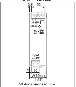
Fig. 21-2 Side view Height: 124mm, 4.88" Depth: 117mm, 4.61" DIN-Rail depth All dimensions in mm
