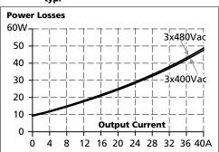
Fig. 11-4 Losses vs. input voltage at 24V, 40A, typ.
