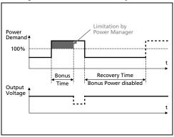
The BonusPower® is available as soon as power comes on and after the end of an output short circuit or output overload.
