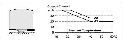
Fig. 24-13 Mounting Orientation D (Horizontal cw)
