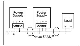
Fig. 14-2 Using distribution terminals
