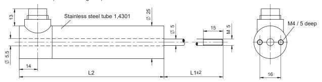
Version with ball joint on plunger (KV) (without rod guide)
