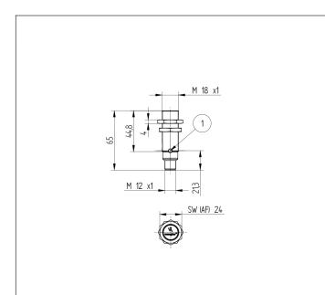
1 = Switching Status Indicator Sleeve M18×1 = 12 Nm All dimensions in mm (1 mm = 0.03937 Inch)
