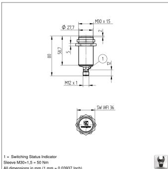
1 = Switching Status Indicator Sleeve M30×1,5 = 50 Nm
