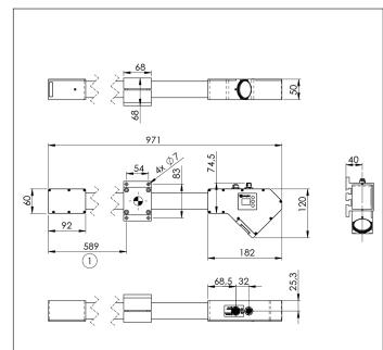
1 = Recommended mounting position based on the sensor's center of gravity All dimensions in mm (1 mm = 0.03937 Inch)
