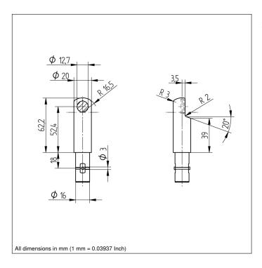
InoxSens is the hygiene series from wenglor. Together with other components, wenglor's InoxSens reflectors in stainless steel protection housing are part of this complete system which is seamlessly integrated into the machine. The reflectors are furnished with IP68 and IP69K protection and are attached using either InoxLock or a mounting console for 20 mm.
